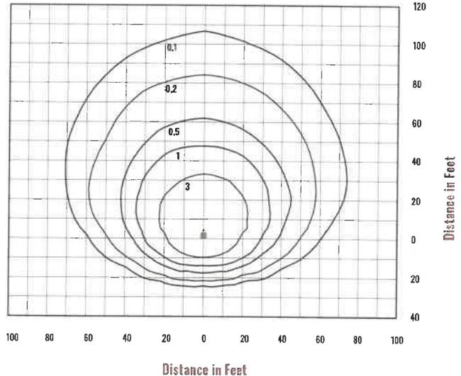
**Note:** All published photometric testing performed to IES LM-79 standards. Fixture photometry was completed on a single representative fixture. Foot candle levels are noted inside graph.
