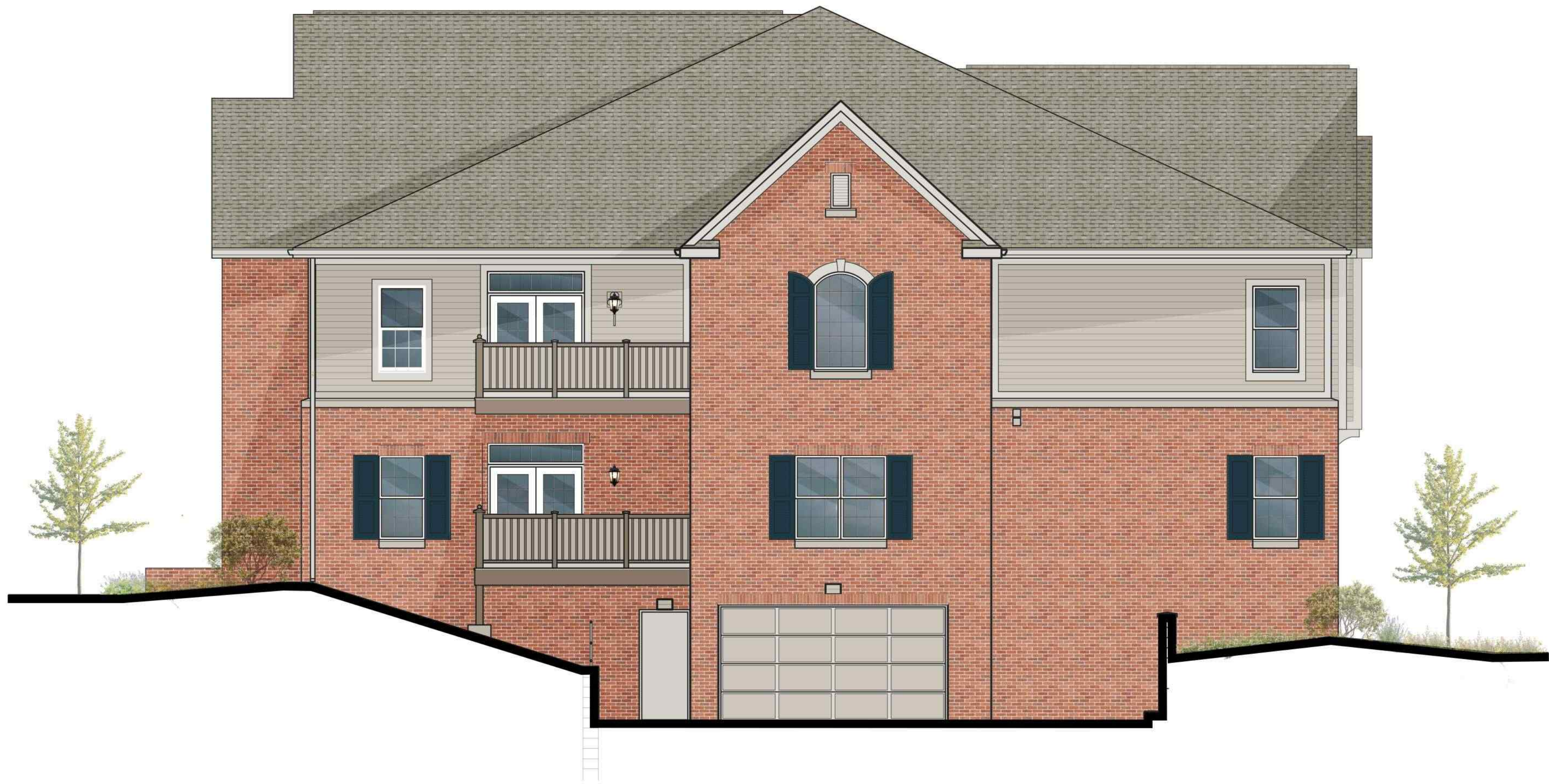
3 RIGHT ELEVATION SCALE: 3/16" = 1'-0"
