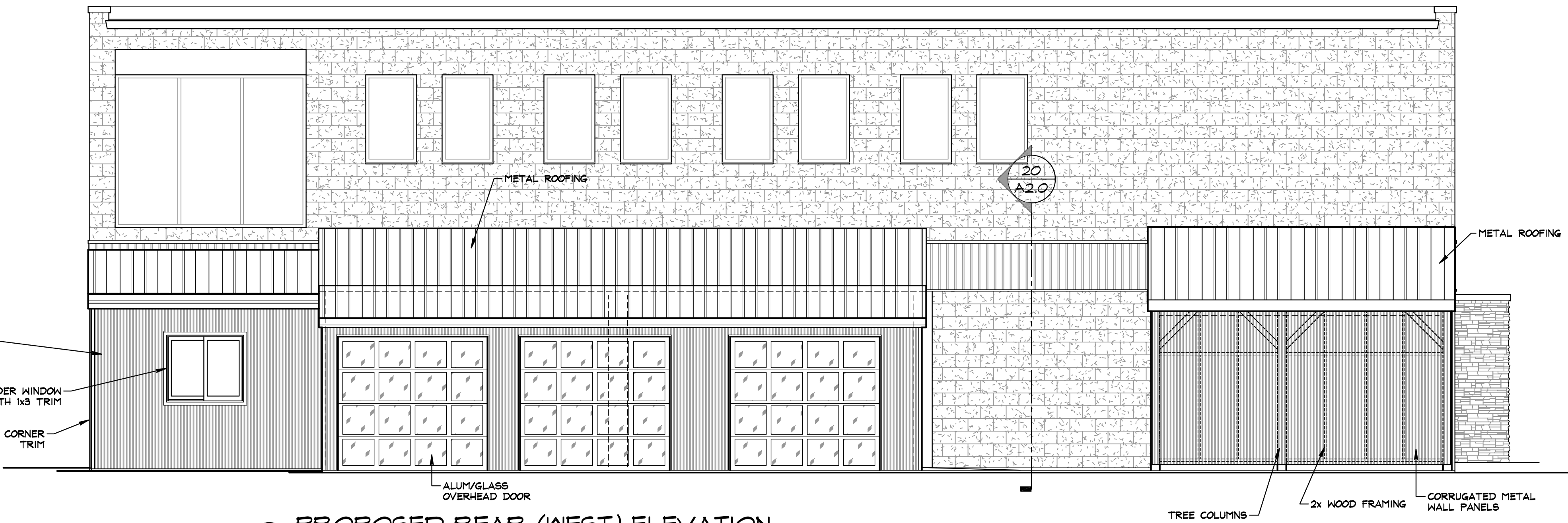
18 PROPOSED REAR (WEST) ELEVATION 1/4" = 1'-0"
